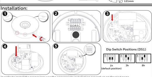
In order to install the proper lens see the appropriate installation procedure on the next page.
