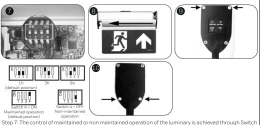
Step 7: The control of maintained or non maintained operation of the luminary is achieved through Switch 4 of DS1. For maintained operation, switch number 4 must be in ON position. For non-maintained operation, switch number 4 must be in OFF position.
