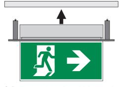
9. Push upwards the base. Make sure that the retaining tags are not expanded.
