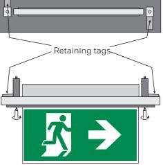
**10.** Fasten the two retaining screws clockwise and the retaining tags will expand until the base is securely installed.
