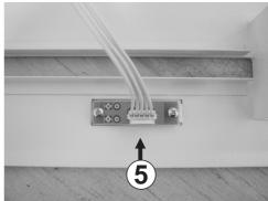
**5.** Install the indications plastic and connect the cable to the respective connector as shown in the picture.
