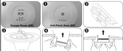
Step 1: In order to place the proper lens (Anti - panic or escape route), first be sure that the luminary is not connected in the mains power supply and the battery is disconnected. A 5 lux lens (Part no. 2900XX.STR) is also available for order. Use the corresponding lens retaining cover depending on the lens you will use.
