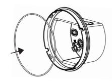
If the Deep Base IP65 option is used, the o-ring seal must be fitted to the base as shown. If required, the deep base gasket accessory can be installed between the base and the mounting surface.
